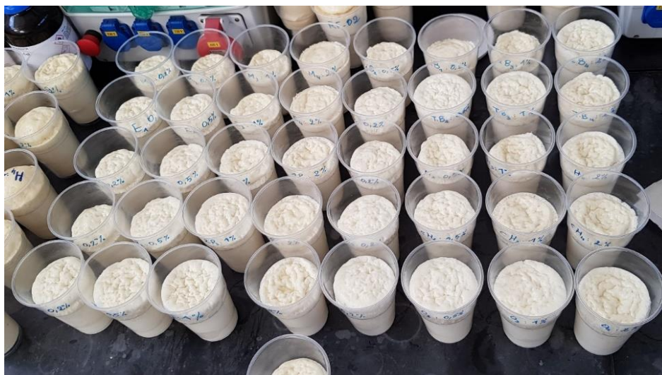
Figure 39: Flexible polyurethane foams, all with the concentration of mono-alcohols at the range of 0.2, 0.5, 1.0, and 2.0%.
