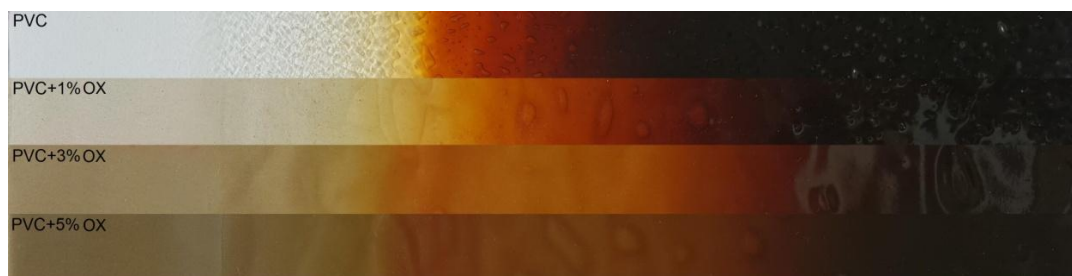
Figure 6. Static heat stability test at 190°C for plasticized poly(vinyl chloride) containing Oxydtron (OX)
