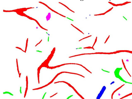
(d) Objects of lamellar graphite cast iron coloured according to their shape
