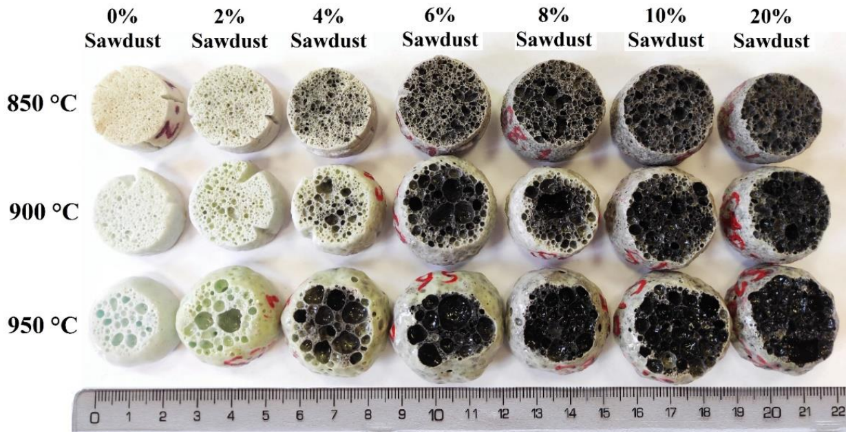
Fig. F. The produced foams with different sawdust content sintered at different temperature
