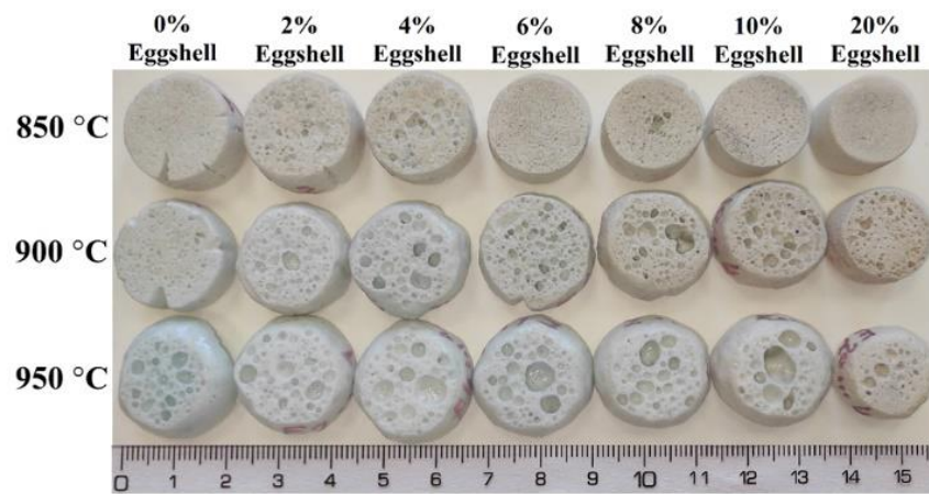
Figure 14. Photos of foamed samples with varied contents of eggshell sintered at different temperatures
